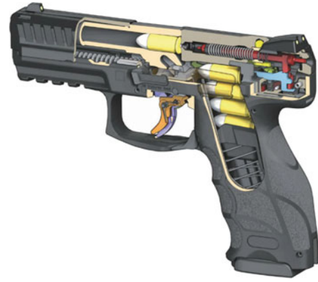
Fig. 3.6 Firearm showing the recoil spring in red [4]
