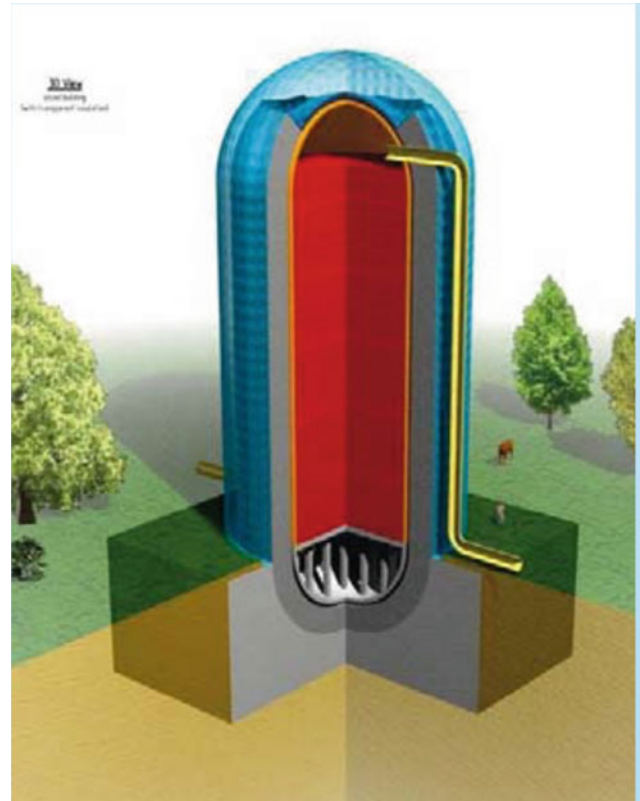
Fig. 9.5 Energy Vault (potential energy storage using gravity)
