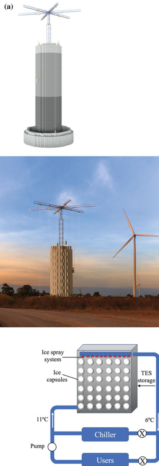
Fig. 9.8 Elements of cryogel ice spray system
